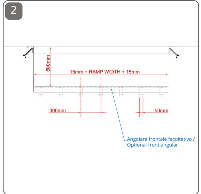
Le zanche devono essere larghe 50mm e distanziate 300mm / The clamps must be 50mm wide and spaced 300mm apart
